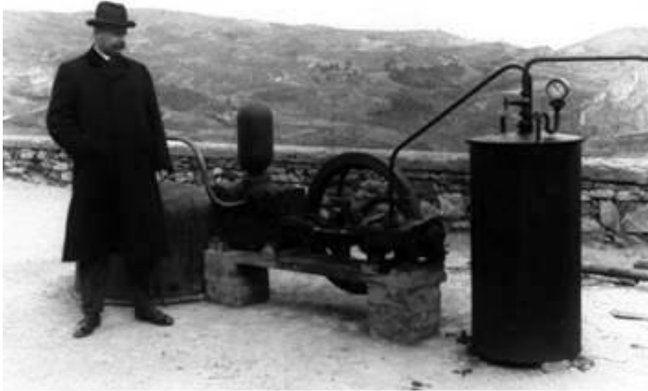
Fig.3 – Lardarello 1904: Prince Piero Ginori-Conti with his apparatus that converted geothermal to electrical energy for the first time in history. (From: UGI 2010)
