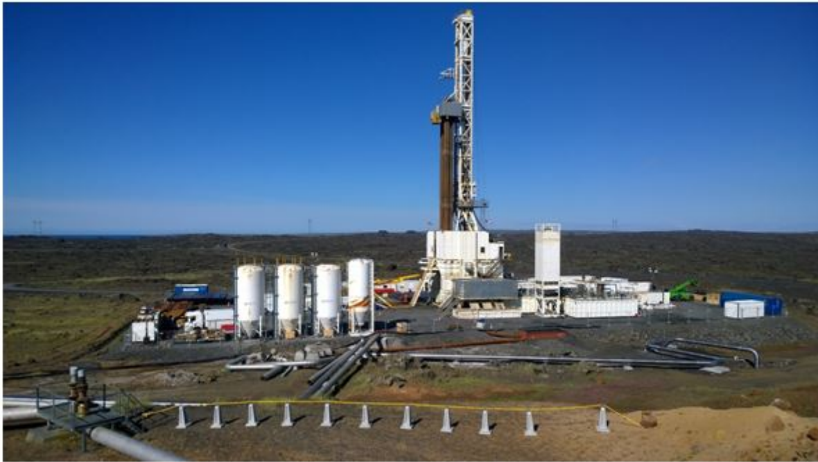
Fig. 1 Geothermal Well at Iceland Deep Drilling Project – IDDP-2 well was completed at 4,659 meters depth searching for a supercritical steam zone
