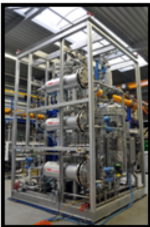
Compact three phase InLine separation test skid
