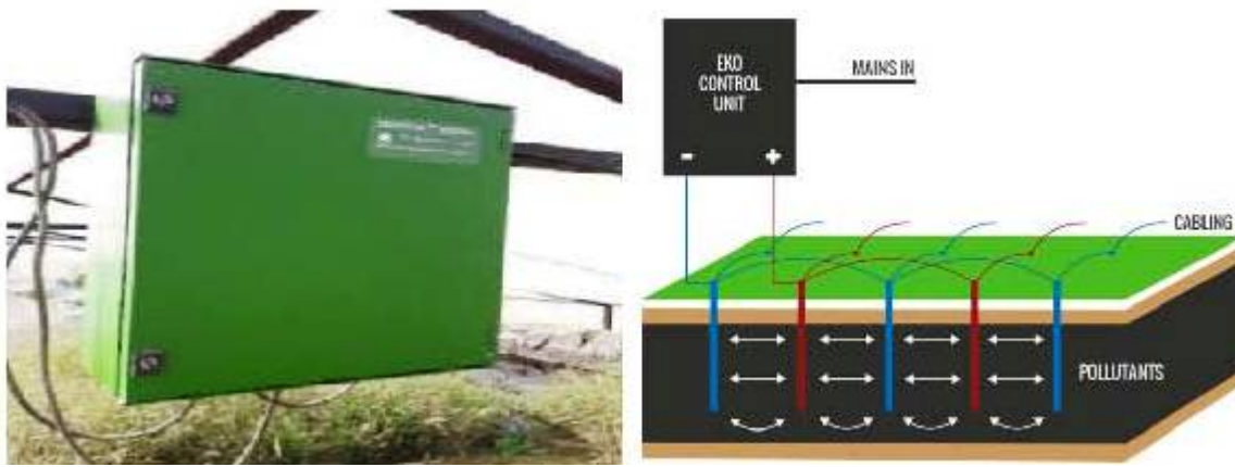
Fig. 4 EKOGRID™ Control unit on a site in Ecuador [5]
